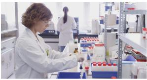
For quality control samples are taken and analyzed according to various criteria. The microbiological examinations are carried out in an external laboratory. From each production batch the return samples are stored accordingly.
